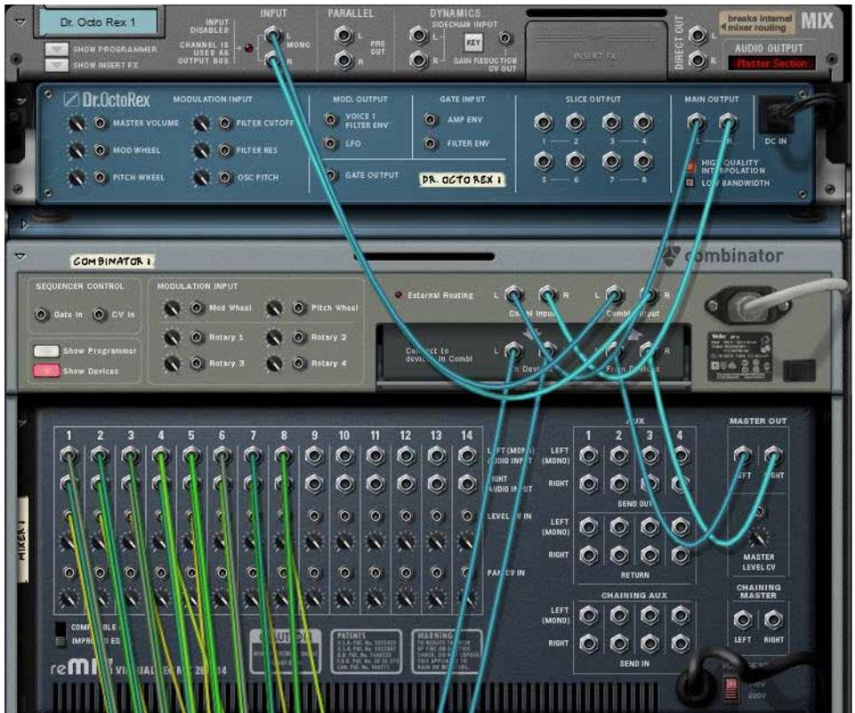
*The routing setup from the Dr. Octo Rex to the Combinator, and the Combinator into Directre (Directre not shown here). This also shows the Audio / CV inputs into the Main Mixer.*
